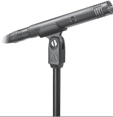
An integral 80 Hz high-pass filter provides easy switching from a flat frequency response to a low-end roll-off. The roll-off position reduces the pickup of low-frequency ambient noise (such as traffic, air-handling systems, etc.), room reverberation and mechanically coupled vibrations. To engage the high-pass filter, slide the switch toward the “bent” line.
