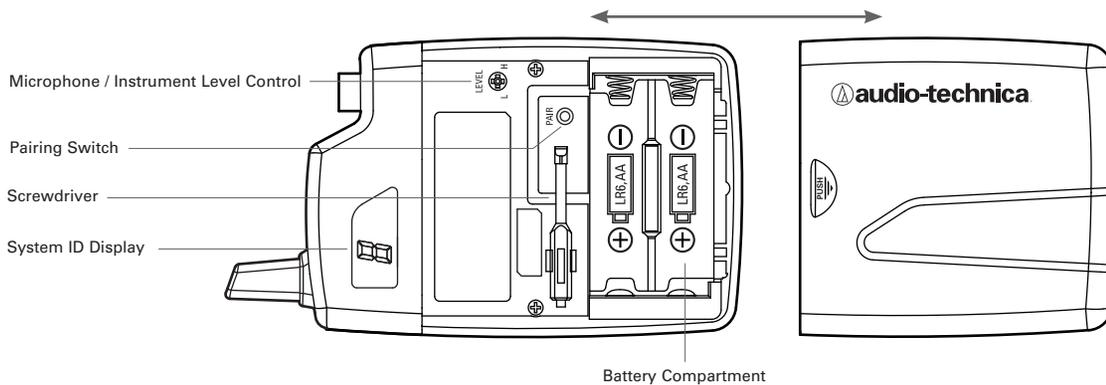
**Figure I – ATW-T1001 UniPak® Transmitter**
