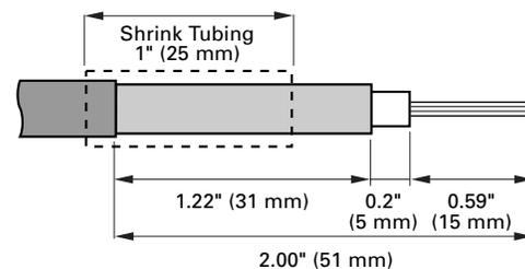
**Fig. E RG8 Cable - Bottom Exit**
