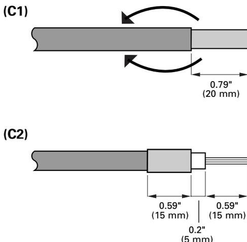
**Fig. D RG8 Cable - Rear Exit**
